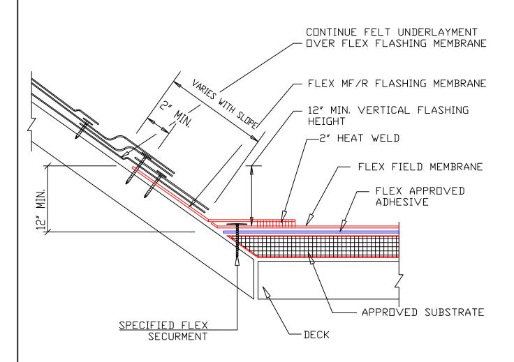
NOTE: THIRD COURSE OF SHINGLES MUST OVERLAP FLASHING MEMBRANE
