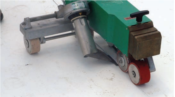
Flex Automatic Hot Air Welding Machine
